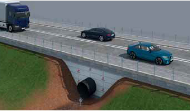
Figure 3 Filling for the purpose of protecting underground pipelines, drainage and infrastructure facilities that are exposed to high vertical load.
