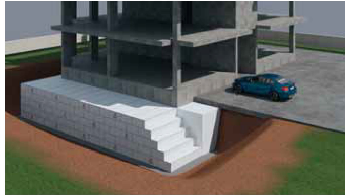
Figure 4 Filling applications for decreasing lateral seismic loads on retaining structures and foundations.
